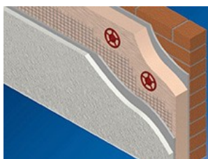
Layers of external wall insulation
